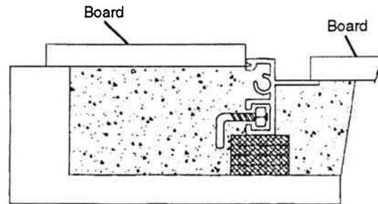
Be very careful that the concrete is absolutely smooth and level with the inside lip of the frame. This will allow the mat to lie perfectly flat and avoid rocking.
