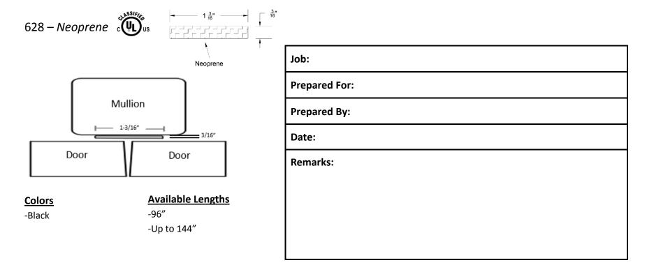
Note: Must be applied on clean, dry frames between 50°F and 100°F. Adhesives have a pre-installation shelf life of 6 to 9 months.
