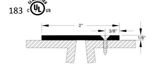
10X1 Phillips flat head sheet metal screws provided. 1/4-20X9/16 thru bolt and screw available upon request.
